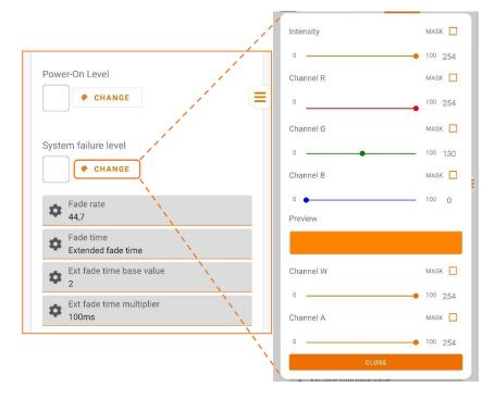
**Power-On Level:** sets the levels of light intensity, RGB, white light, and amber light to which the output is brought as soon as the device is powered. The parameters can be set using the "Change" submenu.
