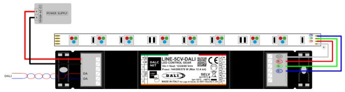
Figure 3: Connection diagram for RGB load
