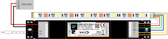
Figure 6: Connection diagram for RGB+WA LED load
