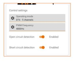
On the *Control Settings screen,* you can configure the different parameters for the driver's operation mode.
