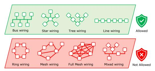
Figure 8: DALI wiring Topologies
