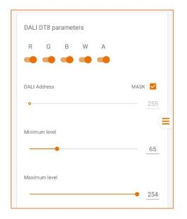
**RGBWA Channel Selection:** individually enable dedicated channels for RGB, RGBW, or RGBWA loads. Depending on the type of load connected to the output, the user can enable the channels used by the LED load.
