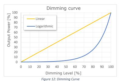
Figure 12 shows the dimming curves supported by the LINE-5CV-DALI dimmer. Curve selection can be done using the Dalcnet LightApp $^{\otimes}$  (see §Control Settings section of this manual).
