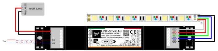
Figure 4: Connection diagram for RGB+W LED load
