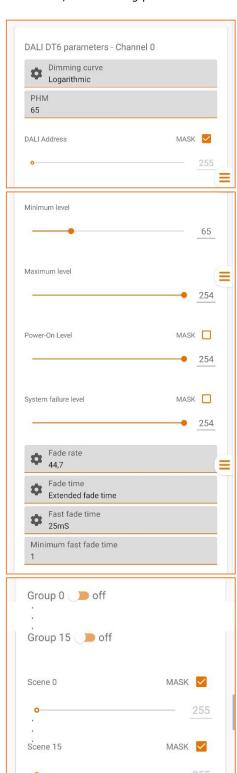
**Dimming Curve**: Sets the dimming curve of the device for operation with remote control. For details on the different curves that can be set, see the §Adjustment Curves section of this manual.
