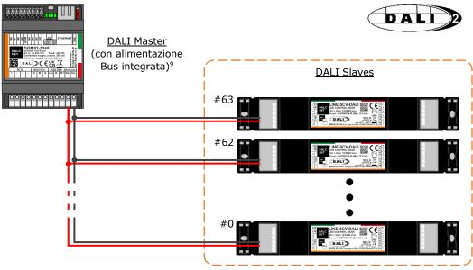
Figure 7: Remote Control Connection Topology, Bus-wiring
