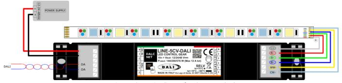
Figure 5: Connection diagram for RGB+TW LED load
